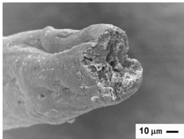
**Figure 5** SEM-image of protein-loaded P(L,D)LA 96/4 filament after 24 weeks *in vitro*.
