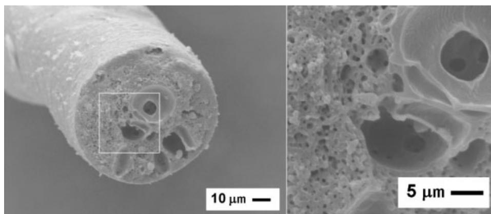
**Figure 2** SEM-images of protein-loaded P(L,D)LA 96/4 filament.
