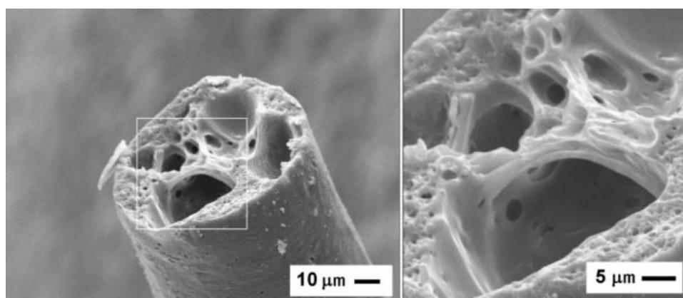
**Figure 3** SEM-images of protein-loaded P(L,DL)LA 70/30 filament.
