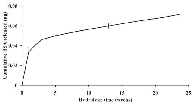
**Figure 7** *In vitro* cumulative BSA released from the protein-loaded P(L,D)LA 96/4 filament.
