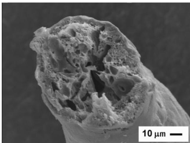
**Figure 6** SEM-image of protein-loaded P(L,DL)LA 70/30 fibers after 24 weeks *in vitro*.
