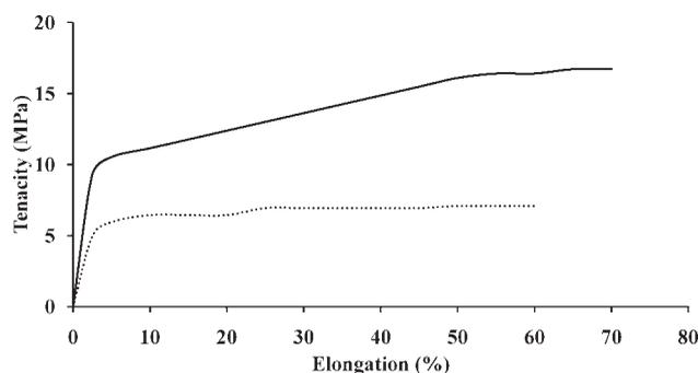
**Figure 4** Stress-strain curves of protein-loaded fibers: (—) P(L,D)LA 96/4 and (···) P(L,DL)LA 70/30.
